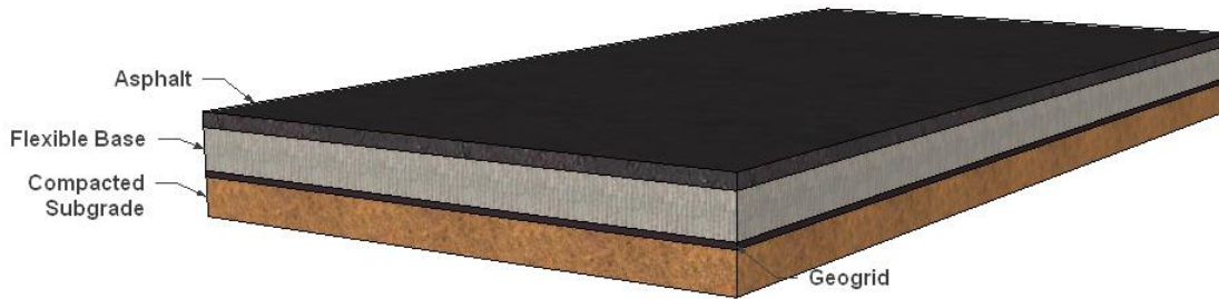
Figure 4.2 – Option 2 Flexible Pavement Typical Section
