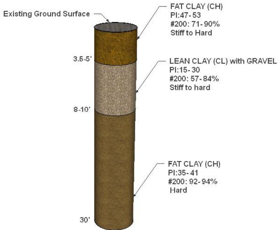
Figure 2.6 – Generalized Subsurface Profile
